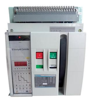
The DW1 series is an intelligent type circuit breaker used to control and protect low voltage electrical distribution network. Possibility to set the parameters of the circuit protection, built in under voltage release, remote control, earth protection and load monitoring.
